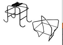
Safeguards pump, gas engine and valves on the job site. Horizontal bars provide convenient hand holds for carrying pump, a pick-up point permits lifting unit with an overhead crane or other device. Standard equipment on PG1203 and PG1204. Can be ordered as an option with any other gas, air, or electrically driven hydraulic pump equipped with a 5-gallon reservoir.
