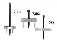
Ideal for pulling many small parts having tapped holes. The 7392 and 7393 may be used with the 1122 pulling attachment to remove bearings, etc. Pullers include two hex head cap screws, 3/8" - 16 NC x 3.00" long. Spread: 1.50" - 4.25". Width of puller block is 4.88". Cap screws are not included with the 522, but any cap screws up to 1/2" diameter may be used. The 522 spread, when used with 1/2" dia. cap screws, is 2"-7 3/4". Width of the 522 puller block is 8.25".
