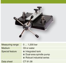
Hydraulic comparison test pump
