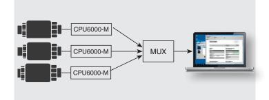
Pressure sensors, model CPU6000-M multimeter, multiplexer and PC with WIKA-Cal software
